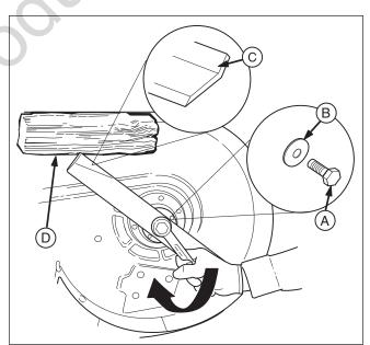
Figure 28. Tightening the Mower Blade for Installation
